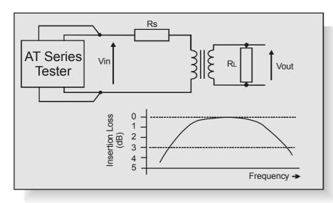
Frequency response is a measure of how the power lost by a transformer (inserted into an impedance matched transmission system) varies with frequency. For an ideal transformer, there would be no power loss. In a real transformer, the power loss increases at low and high frequencies due mainly to the effects of the magnetising and leakage impedances respectively.
