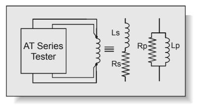
The equivalent ac resistance of a winding may be different to that measured at dc. The resistive part of the complex winding impedance will vary with frequency due to skin and proximity effects.
