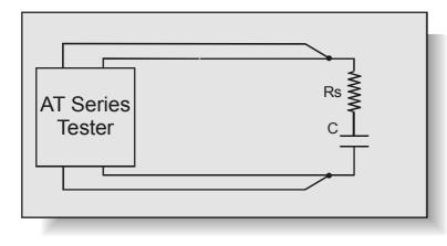
'Dissipation factor' or 'tan $\delta'$  is most often used as a measurement of the losses in a capacitor. It is analogous to 'Q' for an inductor.
