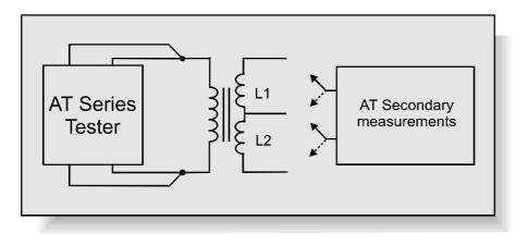
The inductance of a winding is determined by the number of turns and the construction and dimension of the core materials; it may also vary with test conditions such as voltage and frequency. See the LS and LP tests.
