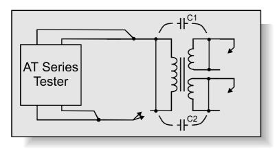
Capacitance occurs in transformers due to the physical proximity of, and electrostatic coupling between, different turns of wire.
