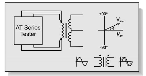
When the ac voltage across one winding is compared to the voltage across another, they may be different in amplitude and phase.
