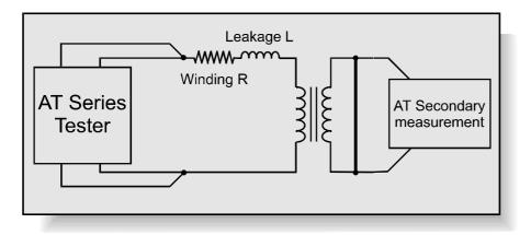
Due to imperfections in the coupling between windings, a short-circuited transformer acts as if there is inductive impedance in series with the winding.
