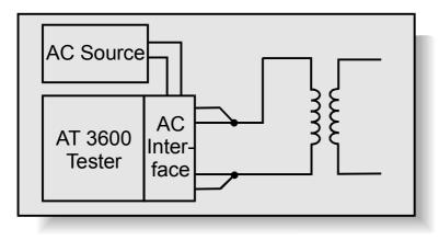
At no load and with its secondaries open circuited, a transformer will still draw current and consume power as described in the WATT test.
