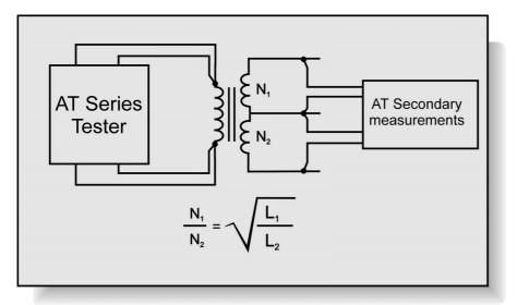
The correct ratio of the number of turns on one winding to the number of turns on another winding is important for the proper operation of any transformer.
