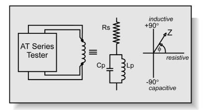
The impedance of a winding is usually complex as it consists of real (resistive) and inductive or capacitive (imaginary) parts. The phase angle  $\phi$ , of the complex impedance at a specified frequency is:
