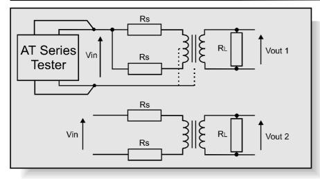
Longitudinal balance is a measure of the common mode rejection ratio (CMRR) of a transformer. That is, the ability of the transformer to reject unwanted noise signals that are common to both input terminals with respect to a common point. An ideal transformer would have infinite CMRR (Vout1 = 0). In practice differences in symmetry of transformer construction mean that input common mode signals appear unwanted as output voltages.
