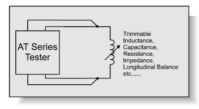
In critical applications, or where the best transformer performance is desired, it may be necessary to trim a particular component parameter to be within desired limits.
