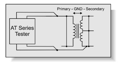
Transformers may be used to provide isolation between dangerous line input voltages and safe low voltage outputs. The transformers may be separate line frequency transformers or power or control transformers inside power supplies and similar equipment.
