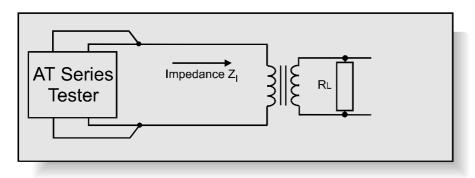
The impedance of a transformer is usually complex, that is it consists of real (resistive) and inductive or capacitive (imaginary) parts. The total impedance at a specified frequency is the vector sum of these parts.
