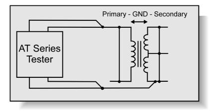
Transformers may be used to provide isolation between dangerous line input voltages and safe low voltage outputs.
