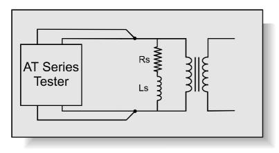
When a transformer is energized, the changing magnetic field in the core causes two types of losses:- hysteresis losses and eddy current losses. The total of these losses can be represented on the equivalent circuit of a transformer by a resistance associated with the inductance of the winding.
