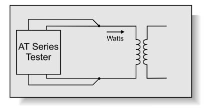
At no load, with the secondaries open circuited, a transformer will still draw current and consume power. The current is typically only a few percent of the normal full-load current, and the  $I^2R$  copper loss is thus negligible. The measured power is then the power dissipated by eddy current and hysteresis effects in the core and is known as the core loss.
