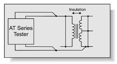
Transformer windings are often insulated from each other and from the core by insulating tape, enamel on the wire or by plastic moulding on the bobbin.
