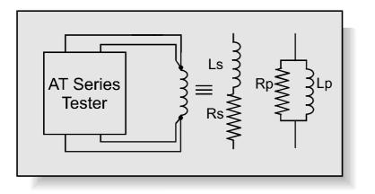
Inductance is the electrical parameter that is commonly used to check that a high frequency transformer has been constructed according to its design and that it will operate properly in use.
