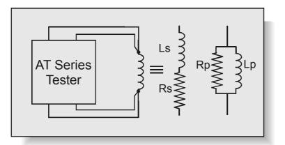
Inductance is the electrical parameter that is commonly used to check that a high frequency transformer has been constructed according to its design and that it will operate properly in use. As well as operating with ac signals, some transformers and chokes are designed to operate with a dc bias current flowing in a winding.
