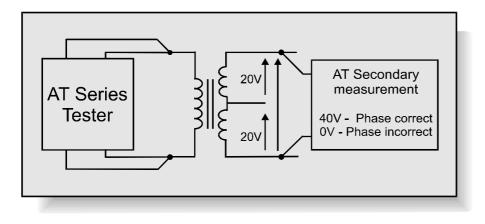
Open Circuit Voltage (VOC) is the voltage appearing across a secondary winding when the primary is energized at a specified voltage and frequency, with the secondary at no load.
