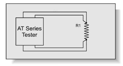
R1 represents the resistance of the copper wire used to wind the transformer. When current flows in the winding, the resistance causes losses in the winding (I<sup>2</sup>R losses), which cause undesirable heating within the transformer.
