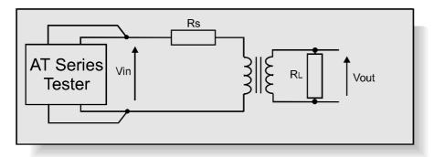
The insertion loss is a measure of the power lost by a transformer relative to the maximum theoretical power that the transformer could transmit to a given load. Core and winding resistance losses mean that some power is always consumed by a transformer, reducing the power
