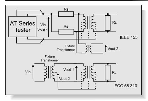
Longitudinal balance is a measure of the common mode rejection ratio (CMRR) of a transformer. That is, the ability of the transformer to reject unwanted noise signals that are common to both input terminals with respect to a common point.
