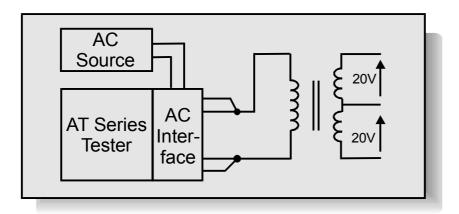
Open circuit voltage is the voltage appearing across a secondary winding when the primary is energized at a specified voltage and frequency.
