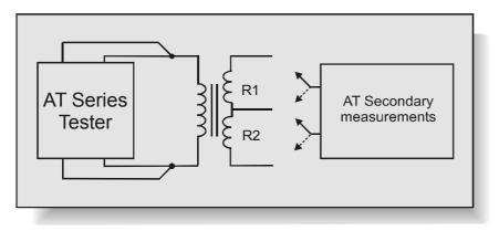
R1 and R2 represent the resistance of the copper wire used to wind the transformer. When current flows in the windings, the resistance causes losses in the windings (I<sup>2</sup>R losses), which cause undesirable heating within the transformer.
